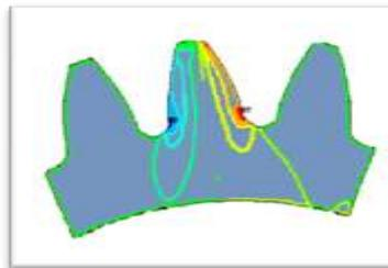
Figure No. 1: Gear tooth bending model
