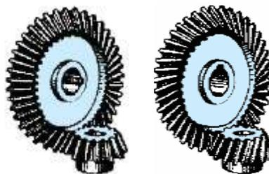
**SPIRAL BEVEL GEAR:** Spiral bevel gears are also used for transmitting power between intersecting shafts. Because of the spiral tooth, the contact length is more and contact ratio is more. They operate smoother than straight bevel gears and have higher load capacity.
