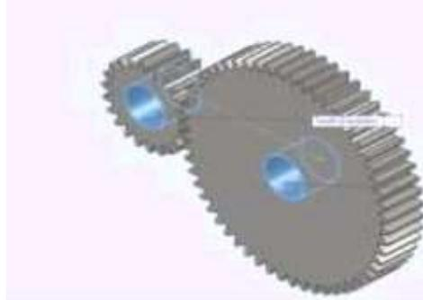
stresses acting on a gear tooth shown in Figure 4.5 are Cross-section =  $t \times b$ , length =  $l$ , load =  $F_t$ , uniform across the face. For a rectangular section, the area moment of inertia is
