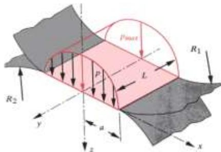
From Figure 3.4 the width of the contact zone is 2a. If total contact force is F and contact pressure is p(x), there is a formula [5], which shows the relationship between the force F and the pressure p(x):
