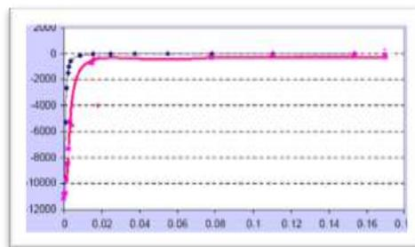
ellipsoidal contact. Note all the stresses have diminished to <10% of  $P_{max}$  within  $y = 5a$  .
